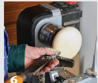
A freshly sharpened scraper produces paper-thin shavings and a smooth surface on the face-turned discs.
