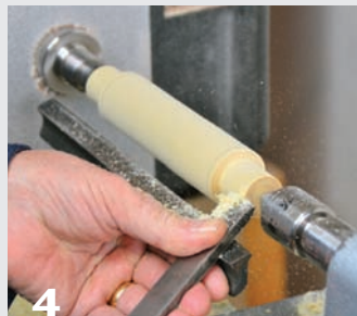
Trim the tenon with a skew chisel. Practice and patience combine for a perfect fit.
