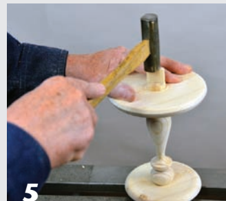
If the tenon is loose, add a narrow saw kerf and tap in a slender wooden wedge.
