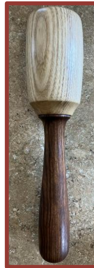
Steve McLoon's dead blow mallet – filled with 1 lb. of lead shot to make it "dead blow"
