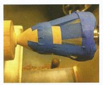
Apply additional strips of masking tape from the top of the cone to the center of your goblet cup. Stretch the tape slightly and secure these strips in place with additional tape applied around the cone and goblet. The purpose of this step is to apply a "pull" versus pushing force on the wood. This will be critical as you begin to turn the stem. This pulling force reduces the tendency to cause "flinging" and/or distortion while turning the stem.
