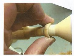
Turn the lathe on at a slow speed. With your fingertips, roll the ring on the revolving sandpaper to shape and finish the inside. The same technique can be used if you want a round ring versus a wedding band style ring.
