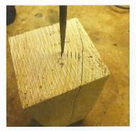
Count the growth rings from the line you just drew to find the approximate center. Mark the same ring on both sides by counting the same number of rings in the same direction on both sides. With an awl or center punch, mark the growth ring you identified.
