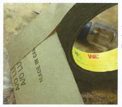
The next steps will prepare a convenient way to finish the underside of your ring. Apply double stick tape to a piece of sandpaper. I use 180 grit.
