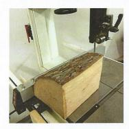
Select a piece of straight, narrow grained wood, clear of any knots or inclusions. Any green wood will work, but a piece that has good grain definition or contrast is helpful. Cut the wood to a 3" x 3" blank, about 7" to 9" long. Try to cut along its grain or growth ring.
