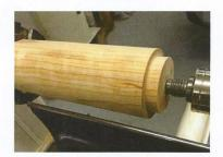
Create a tenon appropriate to the 4-jaw chuck and jaw profile you'll be using.
