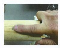
I use a rule of thumb (or should I say "finger") to determine the depth of the cup. Consider a depth that allows comfortably extending your index finger inside the cup for sanding and finishing.
