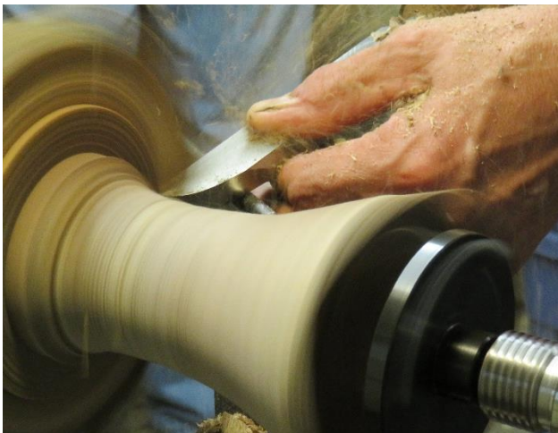
The top was undercut and the stem finished
