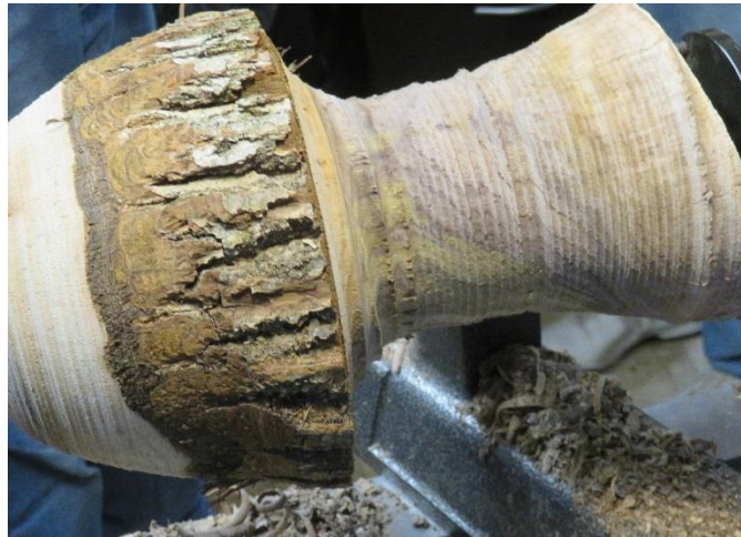
and then roughed out the stem
