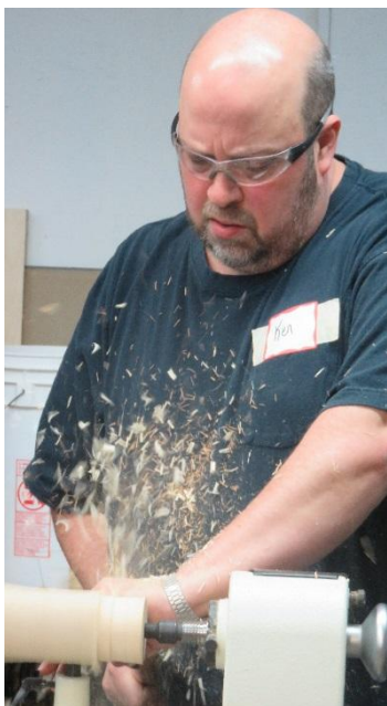
Ken shows that a peeling cut with a skew takes off a lot of wood fast.
