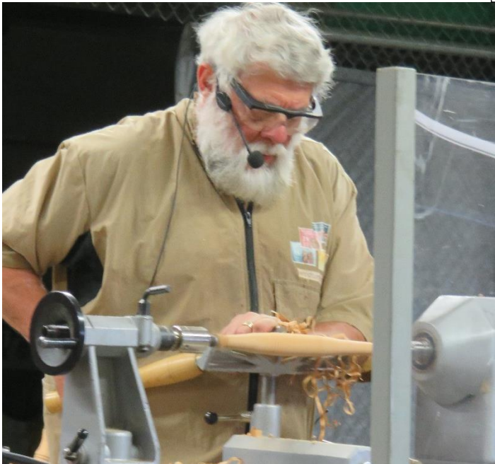
Steve turns stretcher. Both legs and stretchers are made using memory sticks (outside profile drawings) for uniform sizing.
