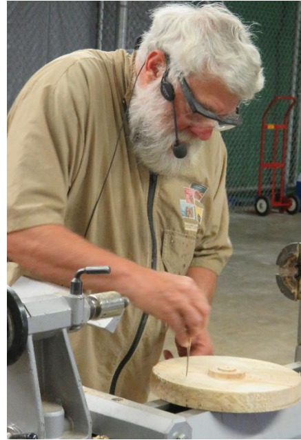
Steve does layout for legs being careful to keep the center of the layout at the center of turning.
