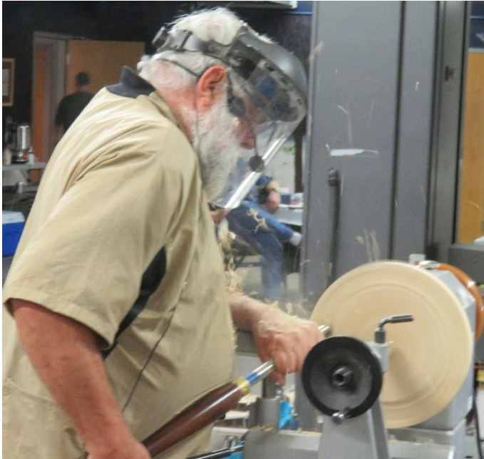
Steve turns the seat with a dip in the center and a radius on the outside edge.
