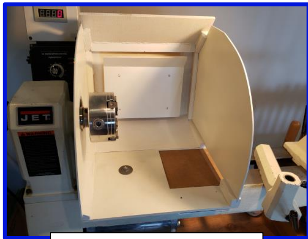
Larry’s lathe-mounted dust collection shroud
