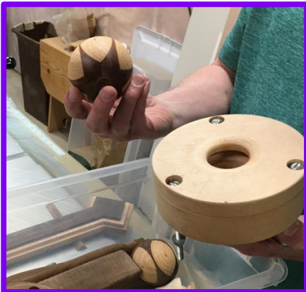
Jay's (Fine Woodworking) jig for hollowing balls
