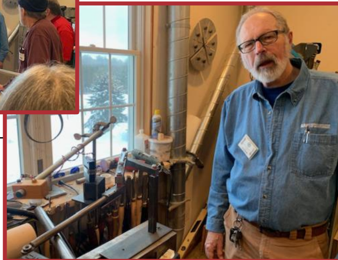
Bob Boettcher explaining his home-made deep hollowing system, with laser light for achieving a desired uniform wall thickness. He's using Paul Keller's rare Australian "Stubby" lathe.
