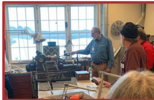
Bob Boettcher explaining his home-made deep hollowing system, with laser light for achieving a desired uniform wall thickness. He's using Paul Keller's rare Australian "Stubby" lathe.
