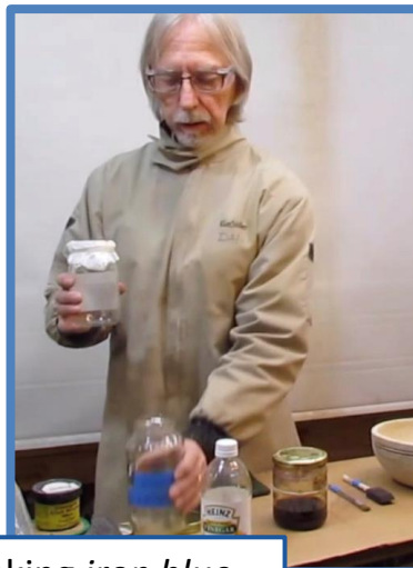
Demonstrating making iron blue stain from steel wool and vinegar
