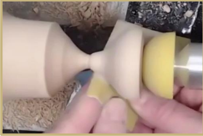
Sanding a cap with canvas backed sandpaper; cap is supported with a "Rubber Chucky"
