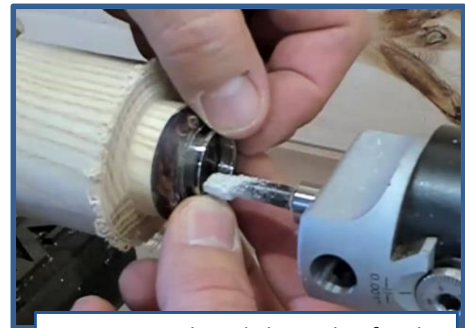
Ring cutter head does the final sizing; trying 1/2 of ring for size
