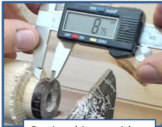
Getting thinner with negative rake scraper
