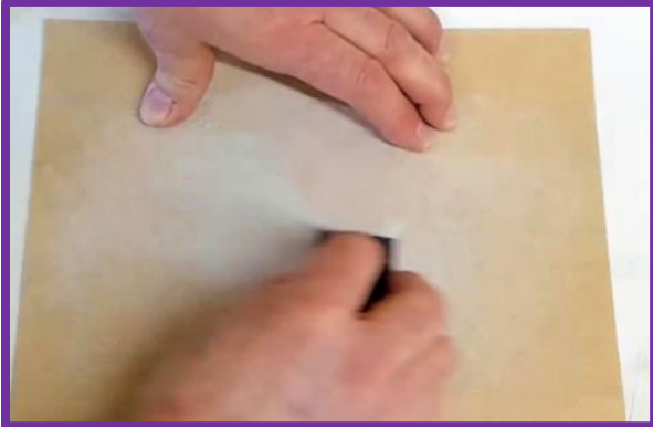
Sanding blank in a "figure 8" manner to flatten for gluing
