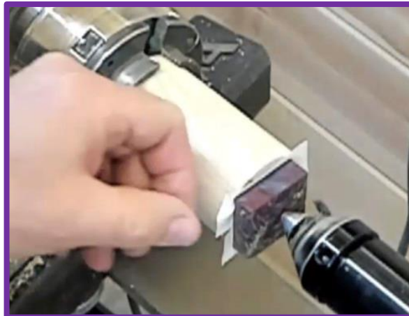
Centering with the tailstock
