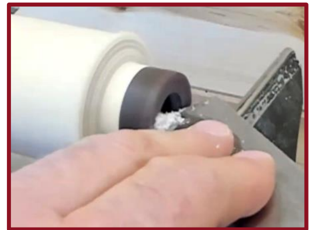
Using negative rake scraper
