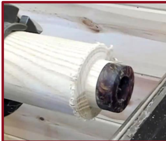
Center of blank drilled out
