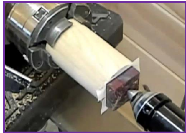
Centering with the tailstock
