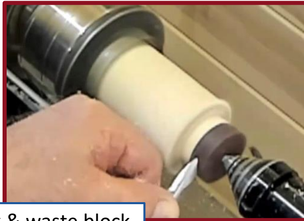
Cutting blank & waste block
