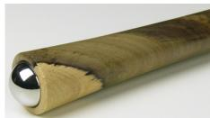
I made this tool handle for Linda (Ferber) sometime back. Part of a flahlight for the ferrule and a steely marble in the handle end.
