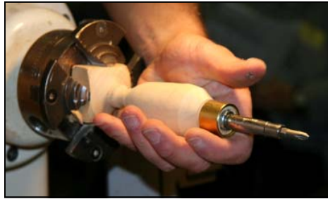
Fig. 12 Dry fit the insert, shaft and collar on the handle
