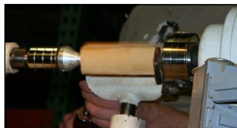
Fig. 4 Turning edges off blank wood
