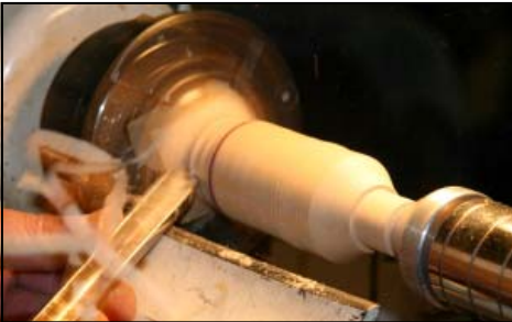
Fig. 11 Heil refined the shape and marked the bottom
