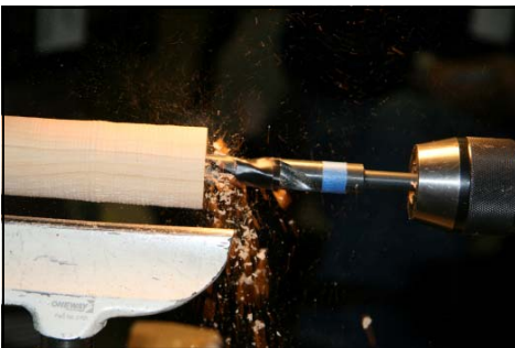
Fig. 6 Drilling holes for insert and shaft
