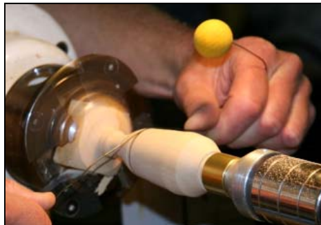
Fig. 13 Wire cutting a groove
