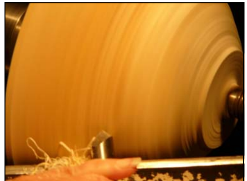
Daves shear "cut" technique virtually eliminates torn end grain .
