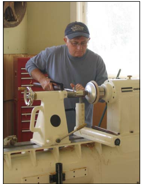
Marv Grabau, working the metal against a wooden form, spins an aluminum bowl.
