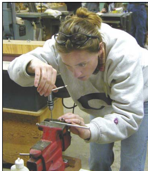
Nancy Sannerud cut threads into a shaft. The threaded hole would house a set screw that would hold a cutting bit in the shaft.
