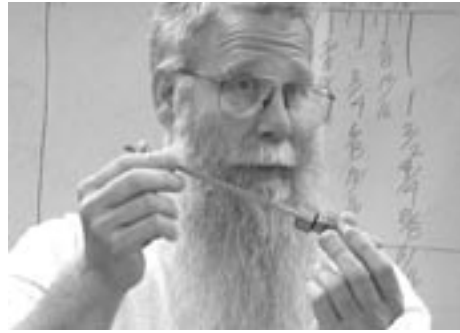
Above, Brad Hubert displays a pen mandrel, an essential tool for crafting pens. At right, a pile of pen blanks that had been drilled and had their brass tubes glued with polyurethane glue.
