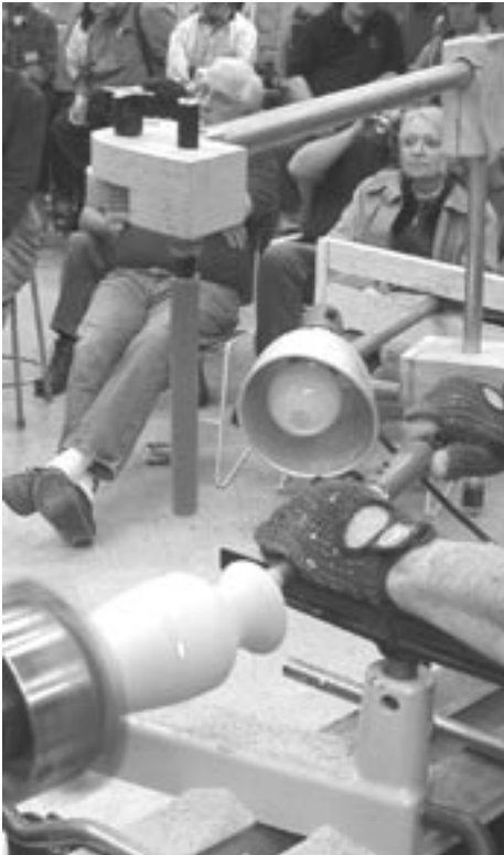
The beam shines on the wood as the piece is being turned. As the wall becomes thinner, the beam gets smaller. When the beam becomes very small and elongated, the wood is very thin.
