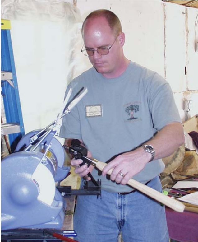
Steve Tiedman demonstrates the Vari-Grind jig that is used with the Wolverine system to achieve the swept back sides on bowl and spindle gouges.
