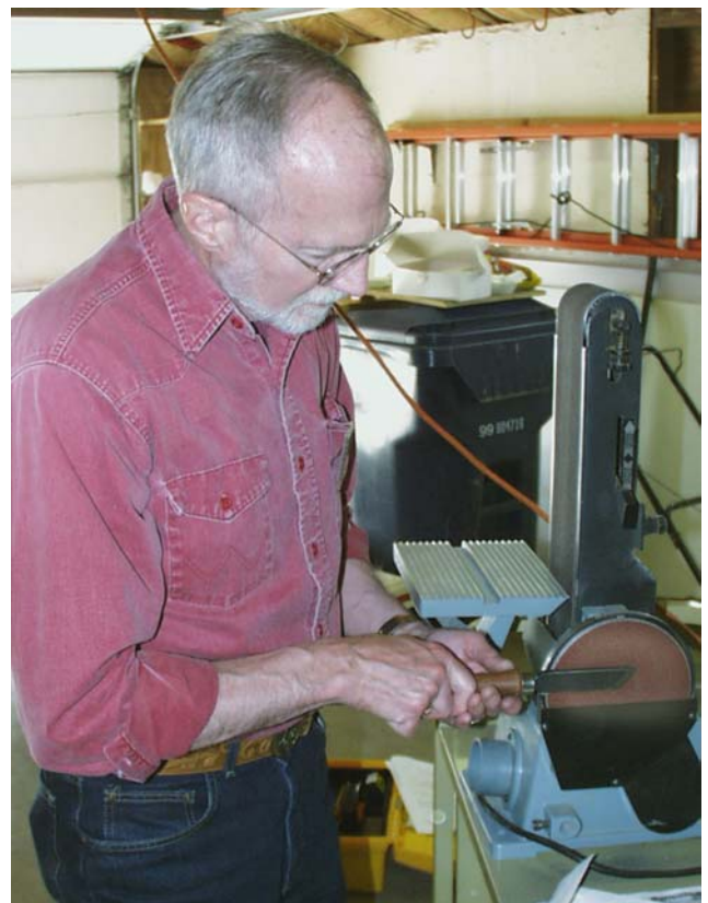
Ken Tempero used Steve's sander to take the sharp corners off his skew chisel before he sharpened the tool. Photo by Chuck Bjorgen
