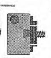
Side view shown with screw center mounted in chuck Reduces the need for many faceplates
