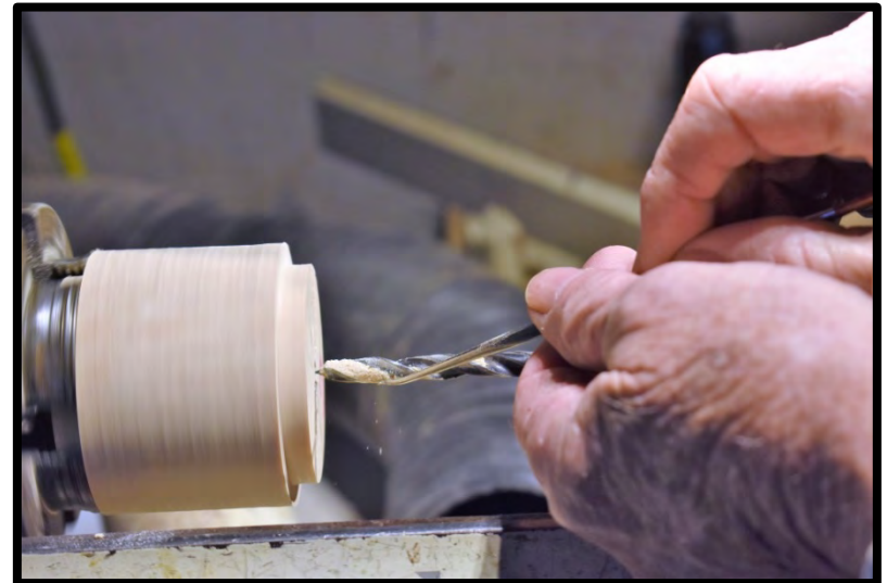
Slide 21 slowly drilling \frac{1}{2} way through while removing wood from drill bit
