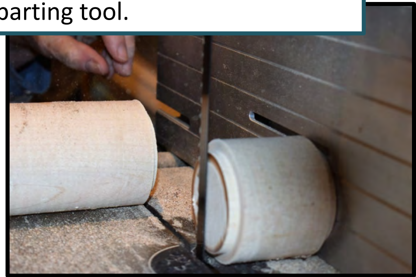
Slide 13 and 13a Cutting PM Top with Band Saw
