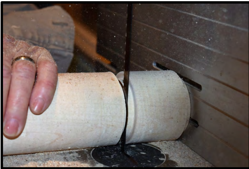
Slide 13 and 13a Cutting PM Top with Band Saw
