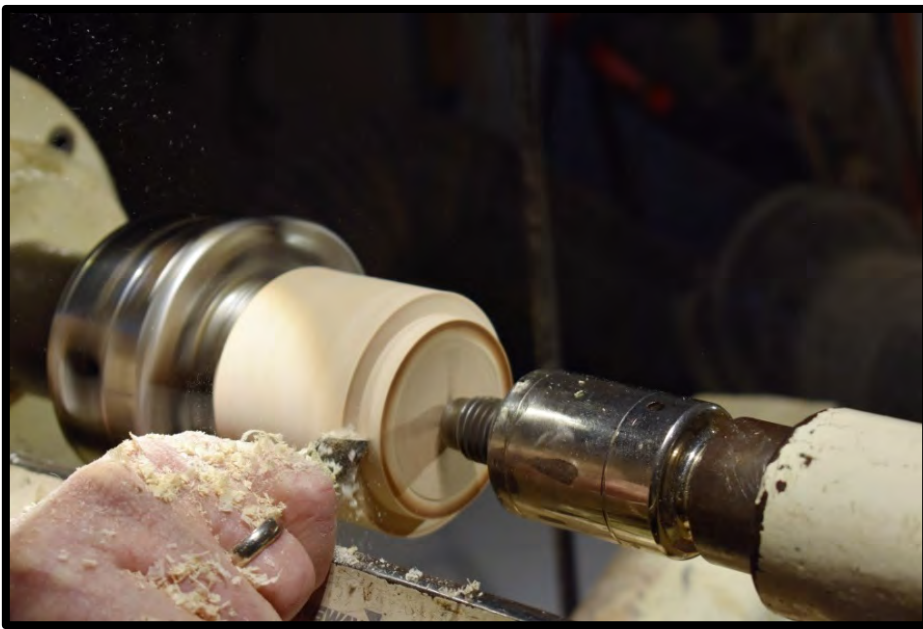
Slide 22 PM Top remounted with bottom facing live center
