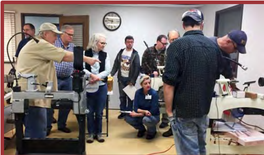
Adjusting the drive belts to change the range of speeds
