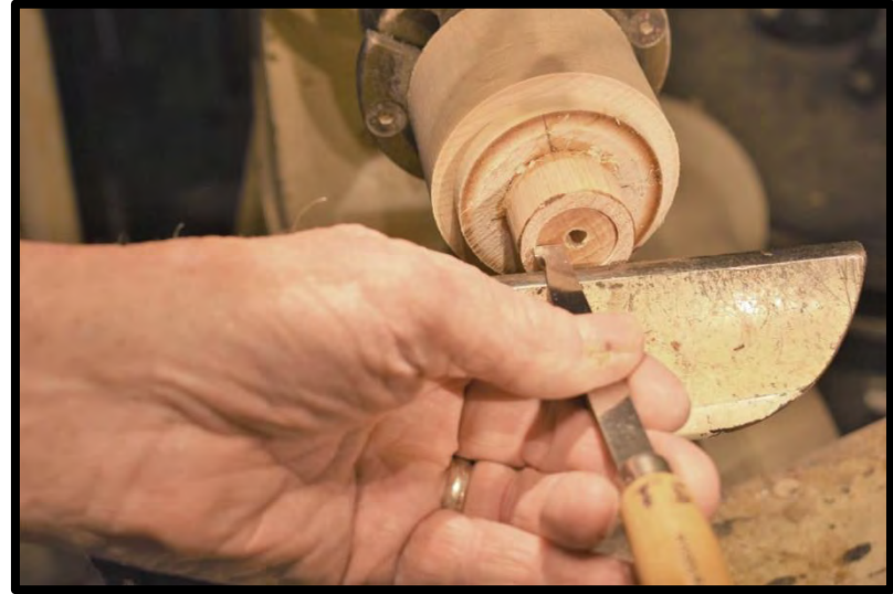
Slide 27 expanding hole to fit 15/32" drive plate
