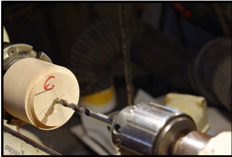
Slide 20 Top remounted, centered and top of PM facing 7mm drill bit
