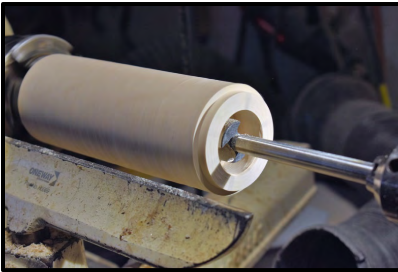
Slide 18 Drilling base with 1- 1/16" bit
