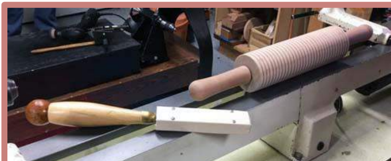
Jim's lefse pin and modified tool with sheath so just the tip is exposed for cutting grooves
