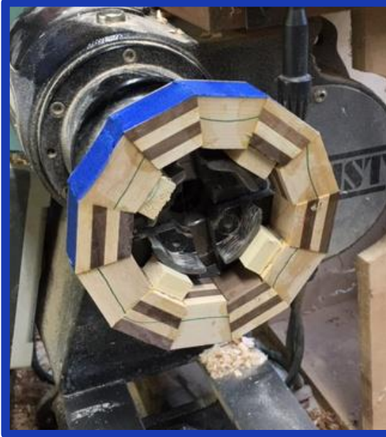
Ring on chuck ready for flattening. Use straight edge to check for flatness. Wood shims may be used if chuck jaws don't expand enough.
