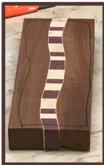
Inlay in segment before mitering
