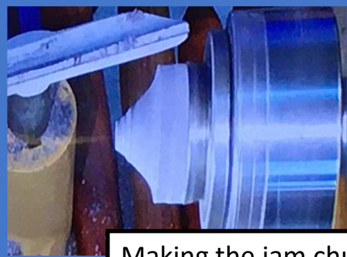
Making the jam chuck after the globe was separated
