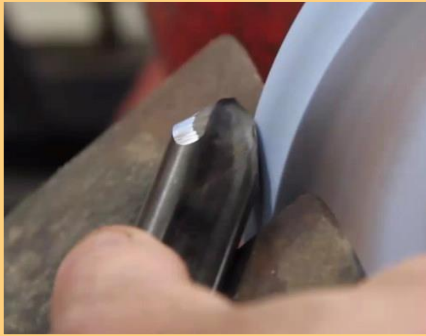
Grinding the gouge by hand
