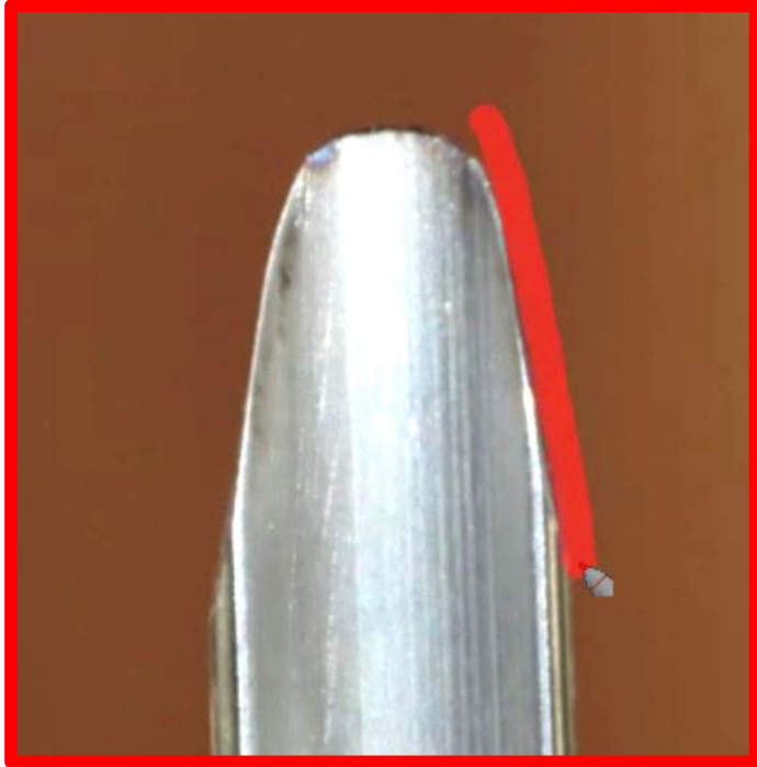
An example of a bad gouge with too broad a tip and NO SIDE metal
