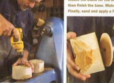
O Drill a center hole in the workpiece. Use a drill bit of a slightly smaller diameter than the screw projecting from the chuck.
