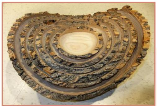
My first 6-piece nested set of an ash crotch. It was dry so I didn't need to have it thicker to allow for warping. Largest with heart is 14 1/2". Now the difficult part, finishing the rough bowls.
