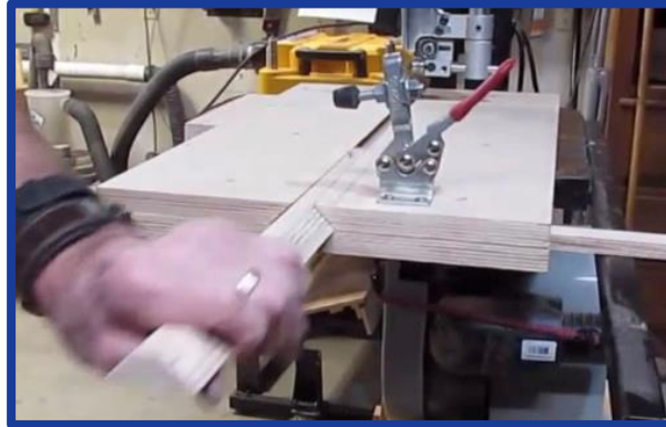
Jig for cutting circles
