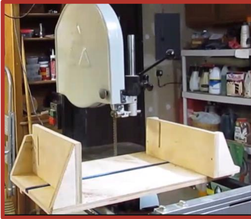
Sled for ripping logs
