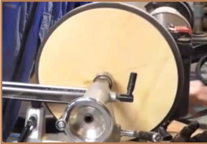
Mounting platter made from 3-4 boards
