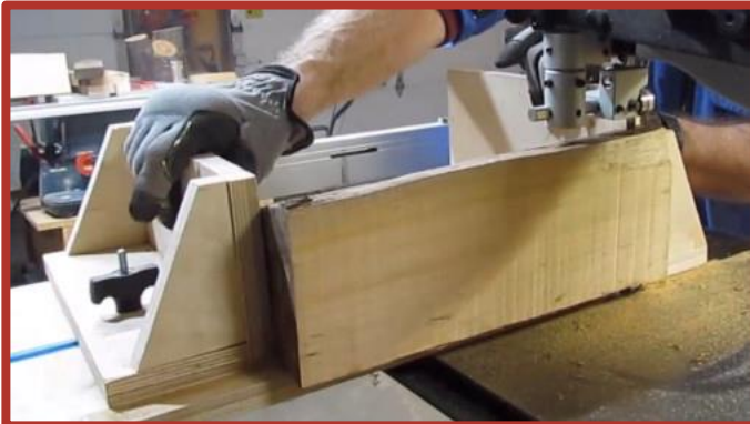
Cutting with sled
