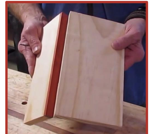
Not glued so the circles can be cut using 2 pieces
