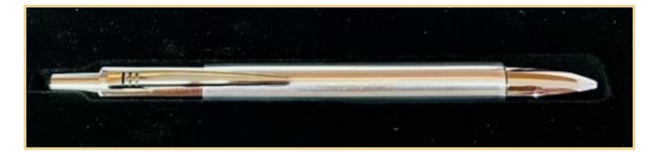
This pen was turned from a solid aluminum billet. Although it contains pen kit parts, the basis of the pen is a homemade design. It has no finish; it is just highly polished.
