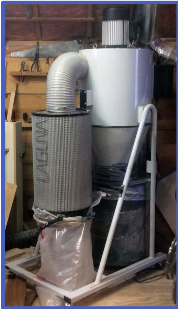
The dust collection unit is in the upper shop and provides collection for both shops
