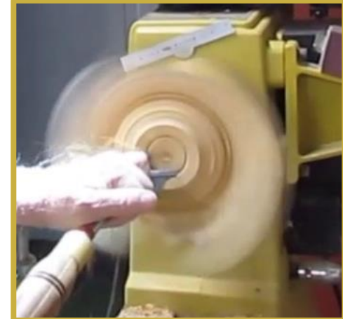
Use 40-degree gouge for the central bulk
