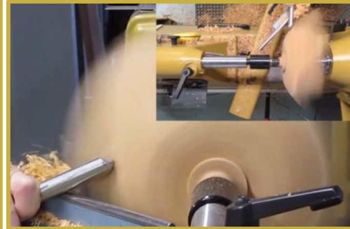
Shear scraping to smooth the bottom
