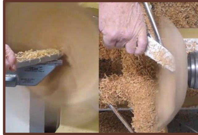
Negative rake scraper to smooth inside
