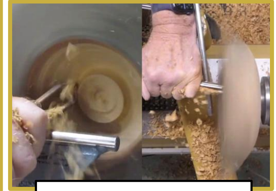
Line up bevel with the outside of the bowl
