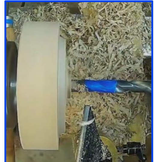
Marking depth of the lid's dome
