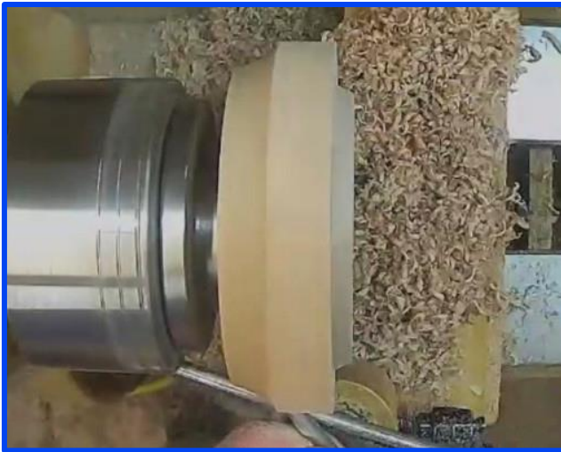
Start shaping the top before it is reversed on the chuck
