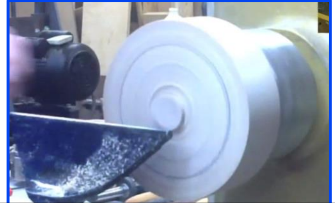
Lid is mounted-width of bottom marked
