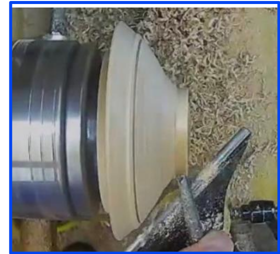
Make a bead on the top and finish the handle
