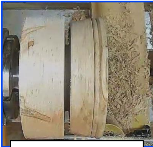
2 beads on the bottom with beading tool
