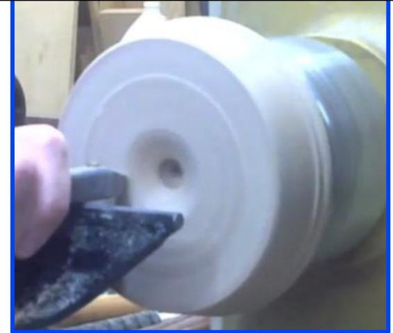
Bottom is reversed on chuck and hollowing begins
