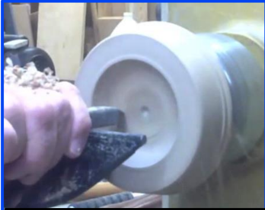
Hollowing continues to the desired thickness of the wall
