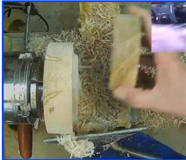
Checking for loose fit with the bottom of the side-grain box
