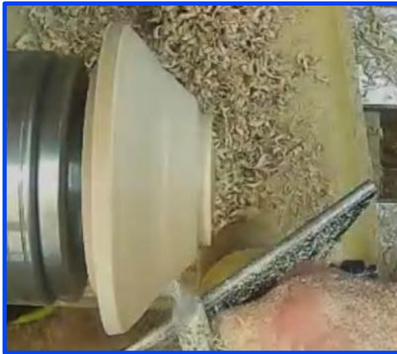
Reverse on the chuck and finish the final shaping
