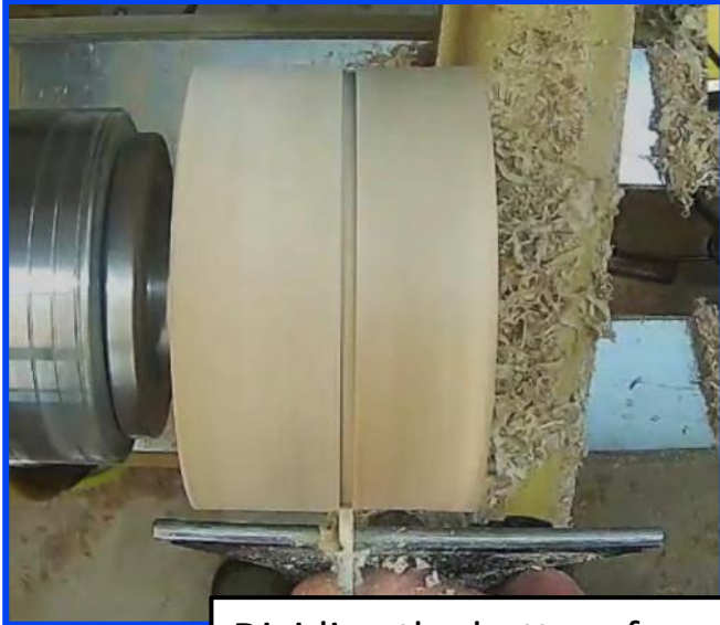
Dividing the bottom from the top of the box blank
