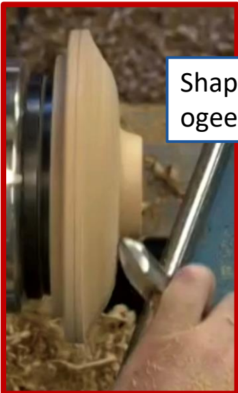
Shaping the inside of the top with the bowl gouge
