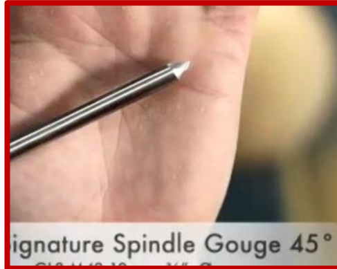
45° spindle gouge with ground off heel for beads
