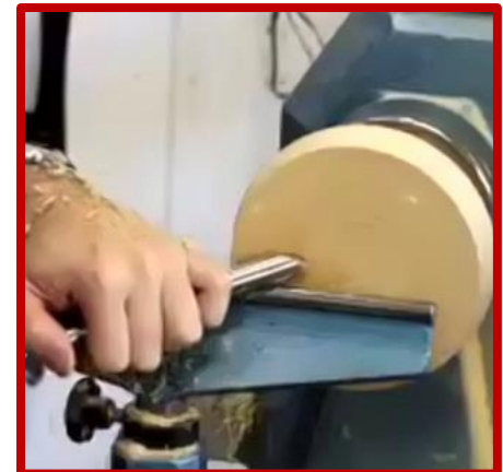
Levelling the top of the base
