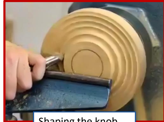
Shaping the knob using push cuts
