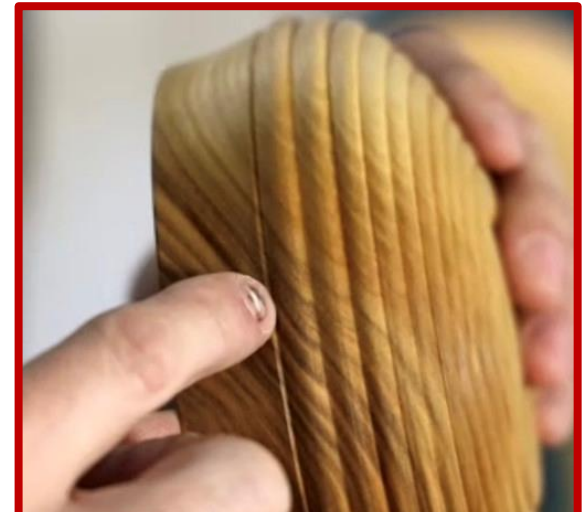
End with a half bead at the concave rim
