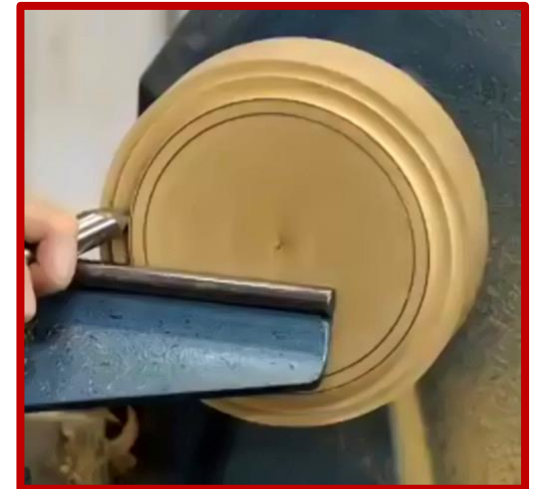
Cutting the lid's tenon
