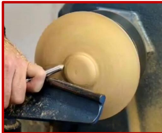
Refining the knob with the spindle gouge
