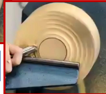
Marking & cutting the tenon
