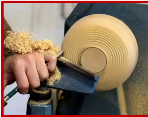
Richard Raffan style bead cutting; keep the angle the same, rock the gouge up and down
