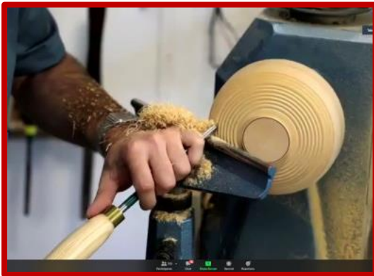
Richard Raffan style bead cutting; keep the angle the same, rock the gouge up and down
