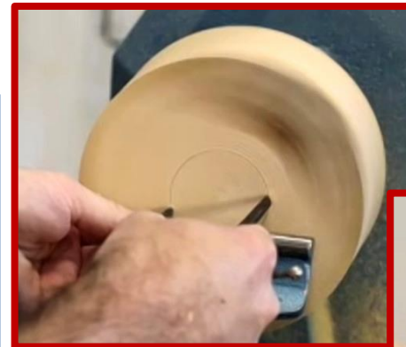
Marking & cutting the tenon
