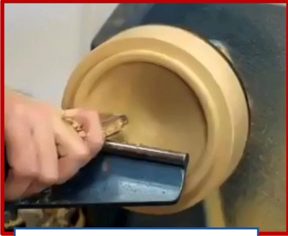
Shaping the inside of the top with the bowl gouge
