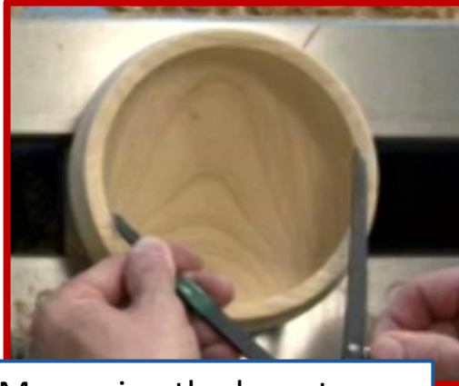
Measuring the base to determine the width of the tenon of the lid; we don't want it tight
