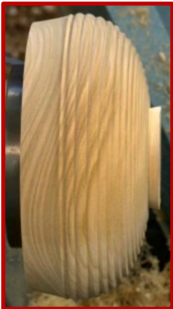
Cutting the concave rim with the 45° spindle gouge and the handle held down
