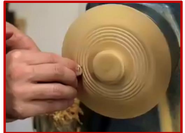
Beads were cut into the lid and are sanded with folded sandpaper
