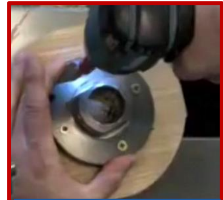
Glenn mounts the base with a faceplate
