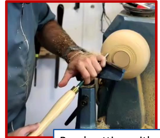
Bead cutting with handle down
