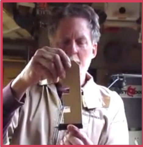
Morse taper jig; bottom is length of the shaft
