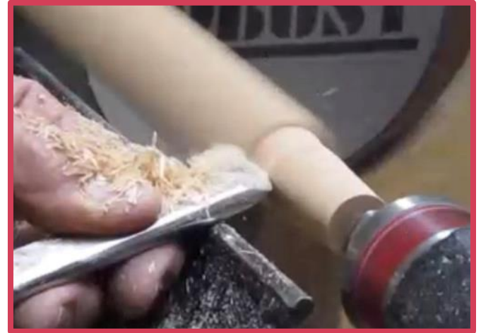
Cutting the Morse taper with the skew
