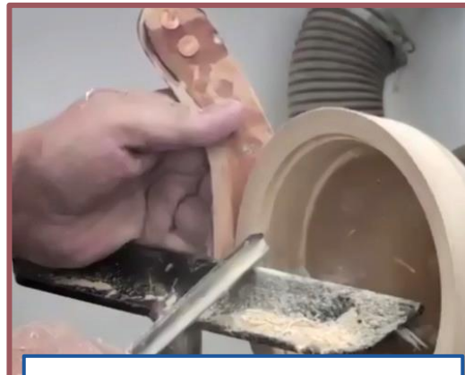
Leather pad to dampen vibration
