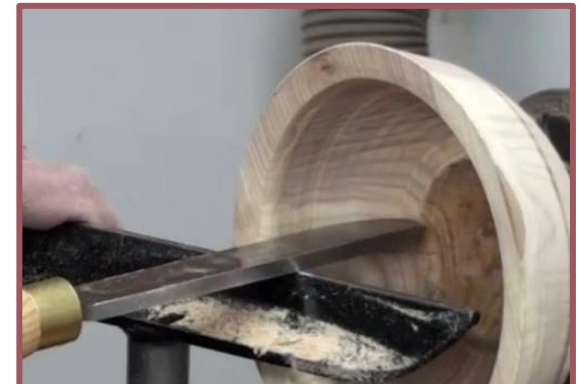
Traditional scraper-cutting edge above center
