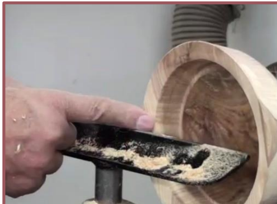
Establishing wall thickness- work down from rim
