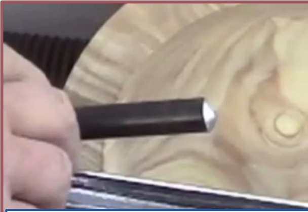
60-degree bottom feeder gouge
