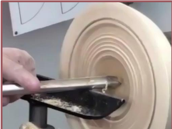
Ledges for rubbing the bevel
