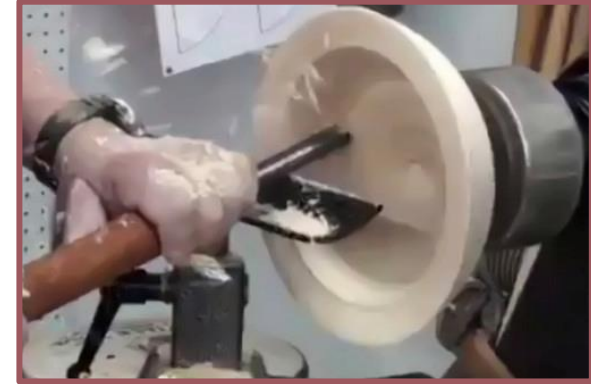
Cutting with the FLUTE UP & LEFT WING of the gouge
