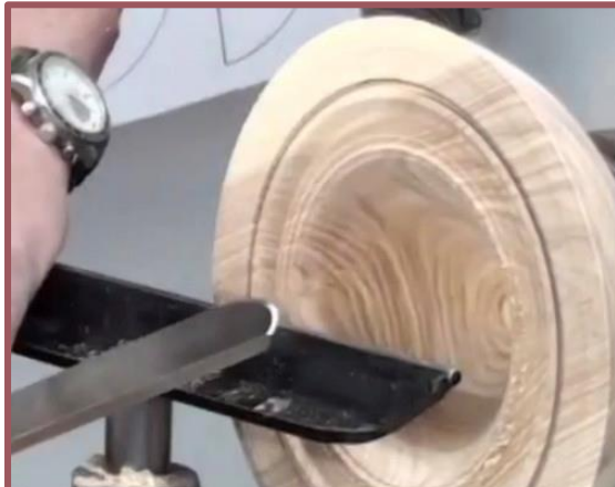
Neg rake scraper for practice
