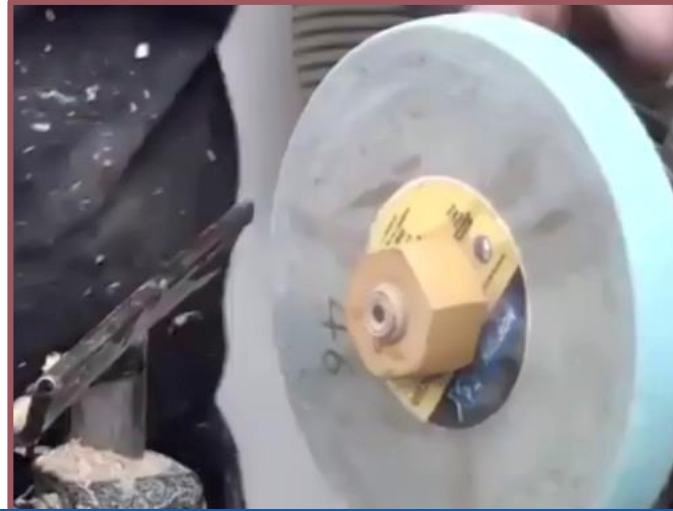
Grinding stone that fits in the chuck
