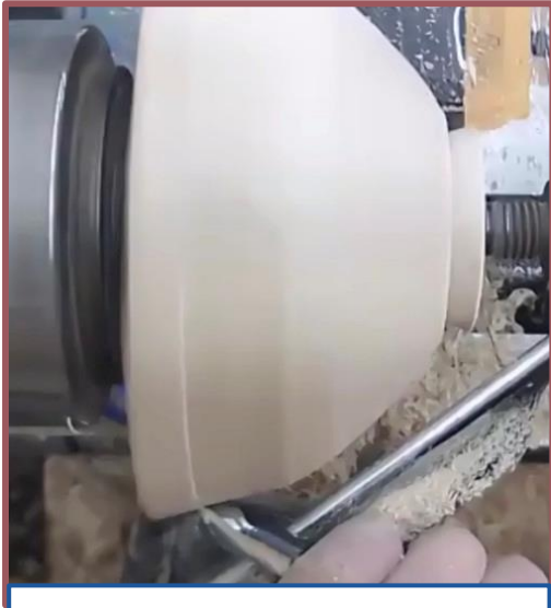
Wrong direction push cut is OK
