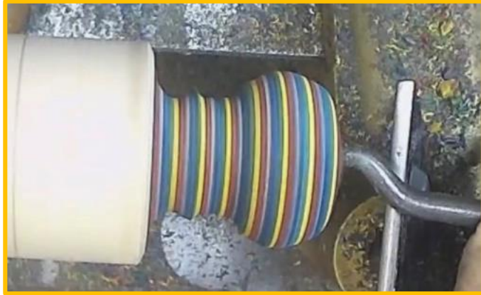
Hollowing with the "back" tool
