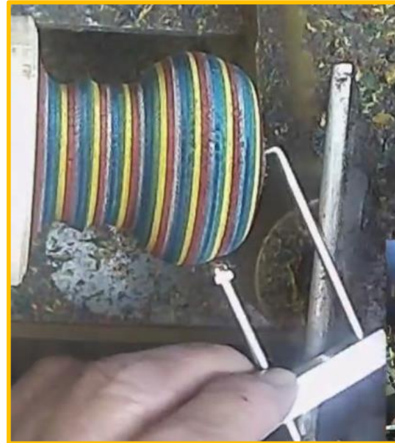
Measuring the wall thickness
