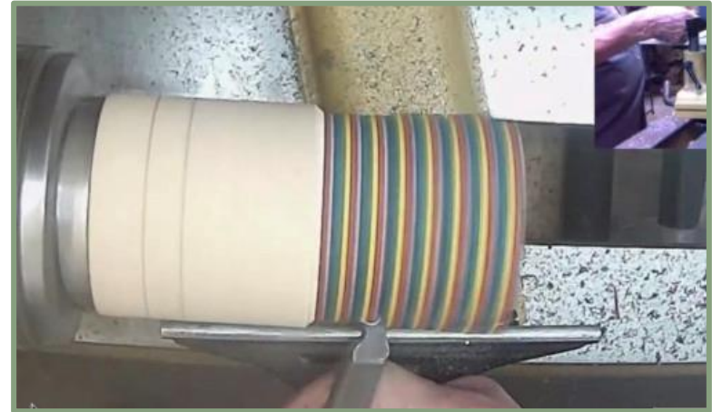
Making a cylinder of a piece of Spectraply. Mike's using a Hunter tool (surprise, surprise!)
