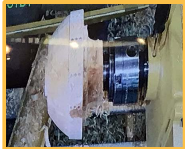
Using Dremel tool to make the pattern of “dimples” on the rim
