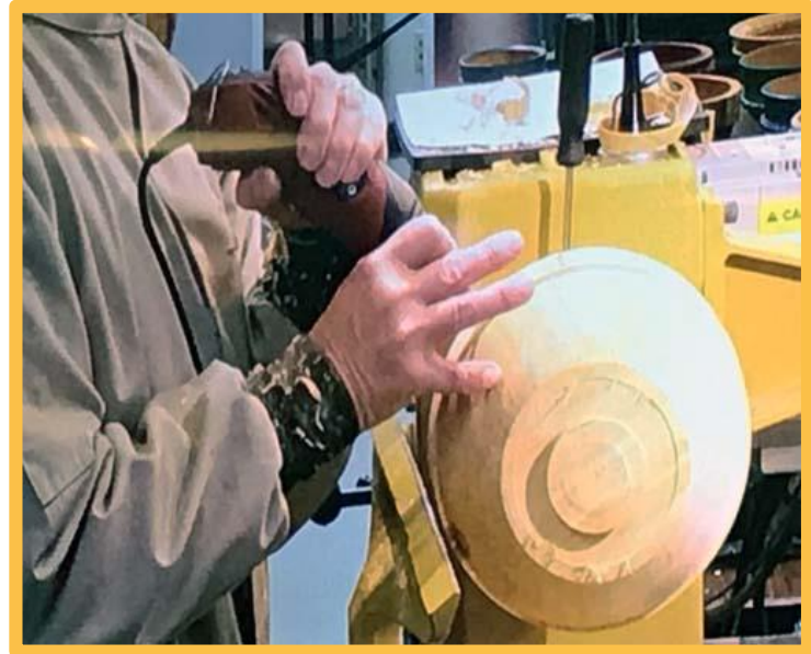
Using Dremel tool to make the pattern of “dimples” on the rim
