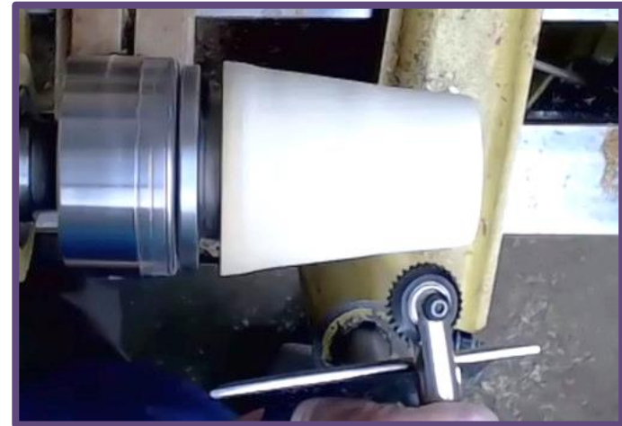
Keep about a 3-finger space between the piece and the tool rest
