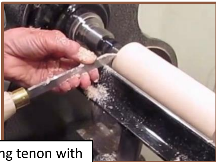
Starting to round the blank with a bowl gouge
