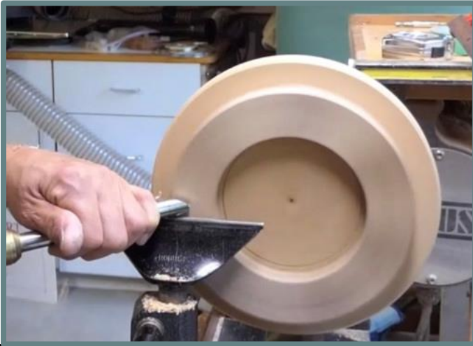
True the ring with LIGHT cuts
