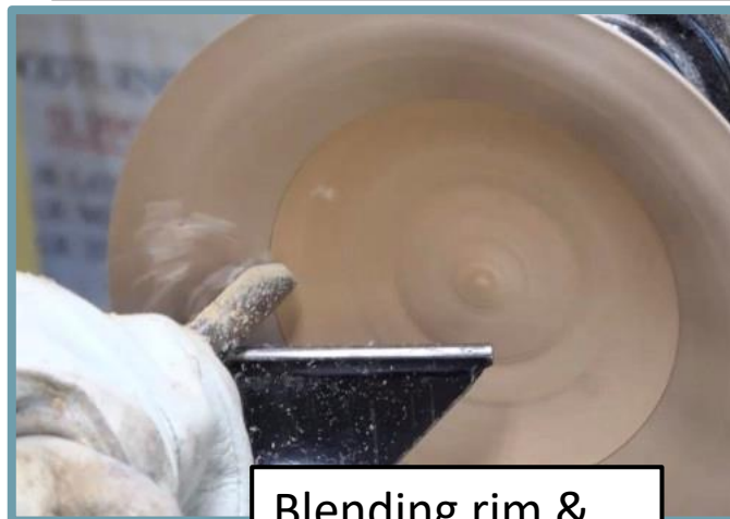
Jim likes the shape of this scraper. Sharpen scrapers UPSIDE DOWN so bur is on top
