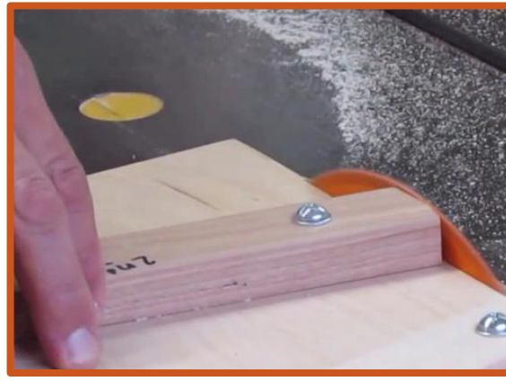
The 1 st cut will trim the edge of the sled
