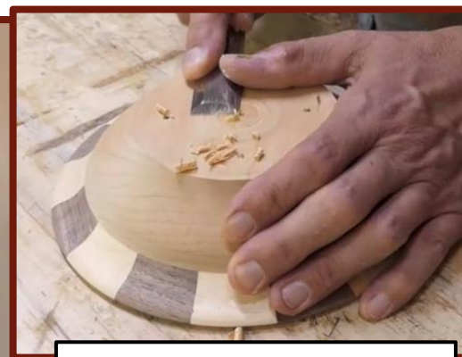
Sharp chisel to remove nubbin
