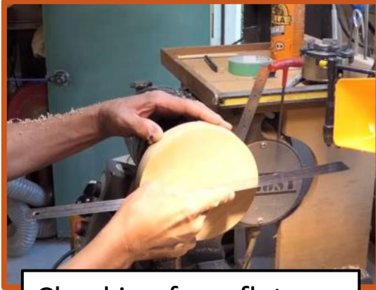
Checking for a flat surface with a ruler
