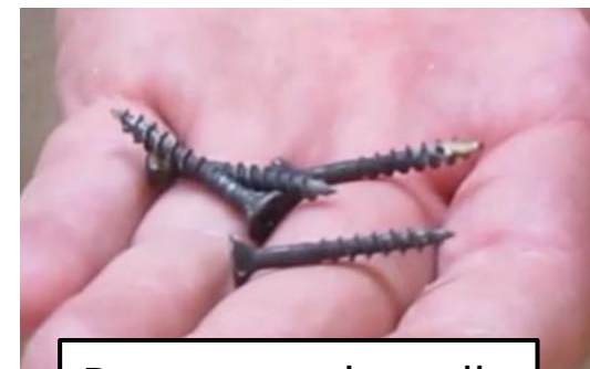
Do not use drywall screws! Use gripper screws like these.
