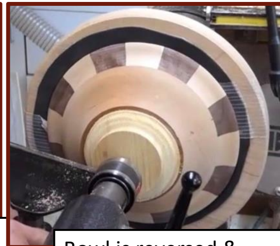
Bowl is reversed & held against foam covered backer board
