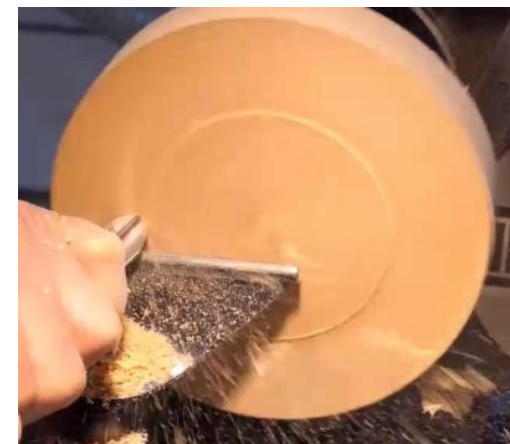
Bevel riding the surface for a push cut
