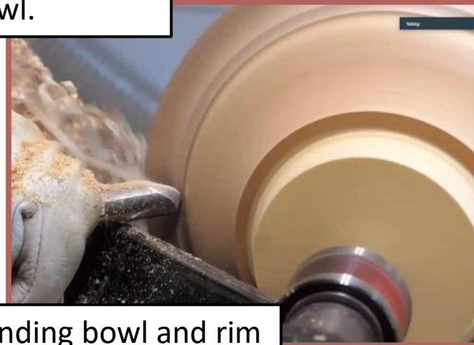
Glue block attached to bottom of the bowl
