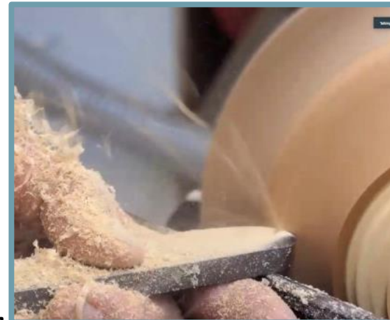
Scraper in action getting FINE chips
