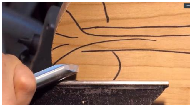
Bowl gouge & side grain-the more open the flute the more aggressive the cut
