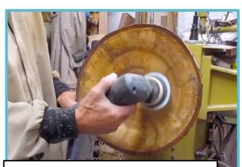
Dan prefers a right-angle drill for sanding. Sand end grain tear out with the lathe off.
