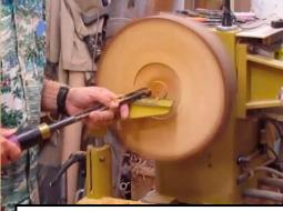
Beginning to make the recess for the chuck
