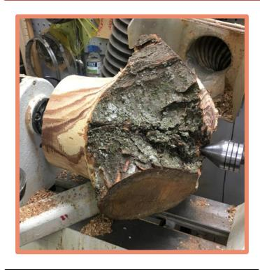
Dan suggested that I mount it and start shaping it like a vase from the base to the top. I flattened the base with the bandsaw and attached a faceplate with screws of adequate length and brought up the tailstock.
