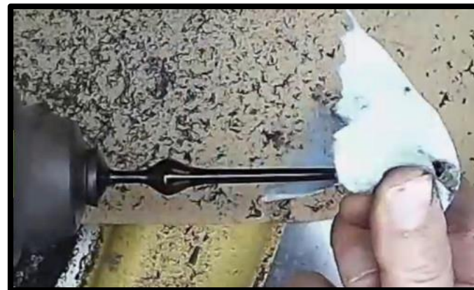
Oiling with walnut oil and generating heat to polymerize the oil
