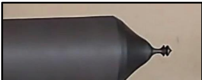
The tip is finished; do 1 section at a time and never go back
