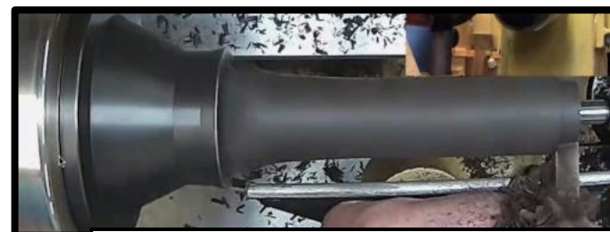
Next, begin the tip; Dick turns at 2500 rpm
