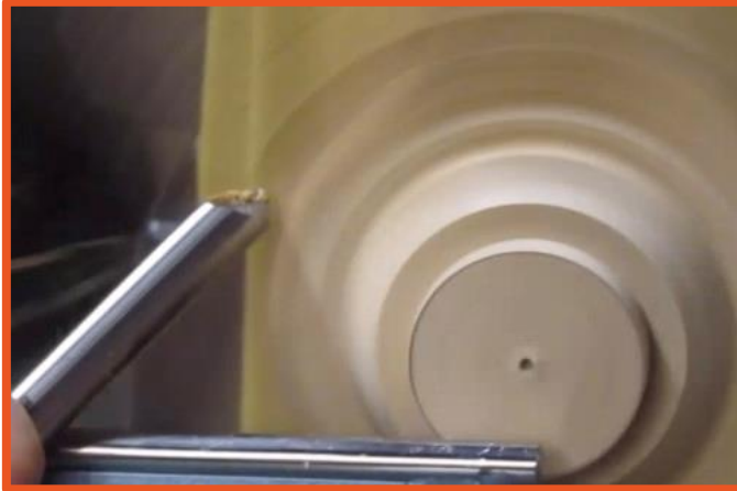
Handle is way down in your pocket. Top wing of gouge "almost" touching
