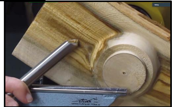
Shear cutting the wing
