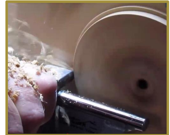
Finishing the junction of the bowl rim and the wing with the skew
