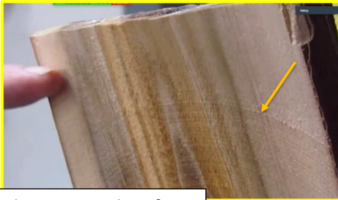
Skew scraped surface above the arrow
