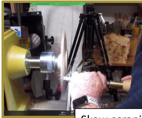
Skew scraping the top of the wing; just very little nibbles at a time
