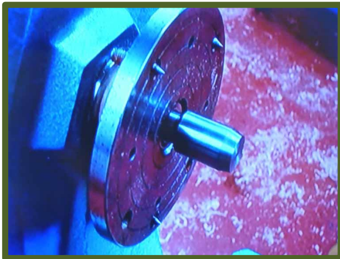
This is a special 6 inch face plate fitted with three bolts ground to a point, with a one inch "post" in the center to stabilize the bowl blank. Faster than a screw chuck in production
