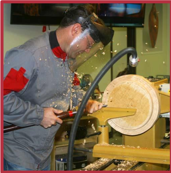
Glenn beginning the platter, doing the bottom first.
