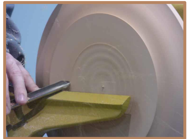
Glen makes the bases of platters and bowls wide enough to be practical, that is, to not tip when in function
