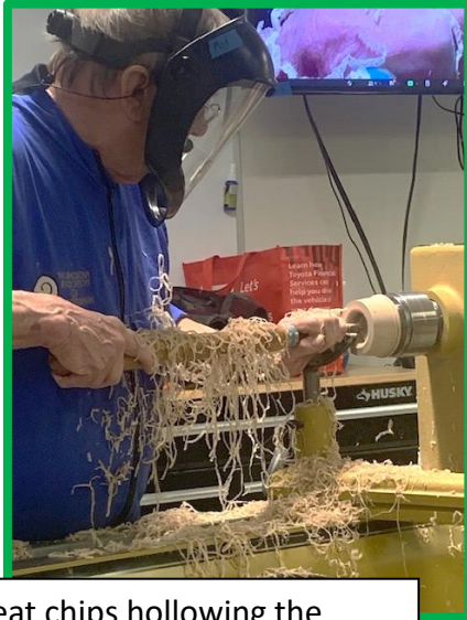
Great chips hollowing the bottom with a Hunter Viceroy
