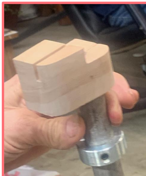
Al Fletcher's jig for cutting rings for bowls from a board in one piece
