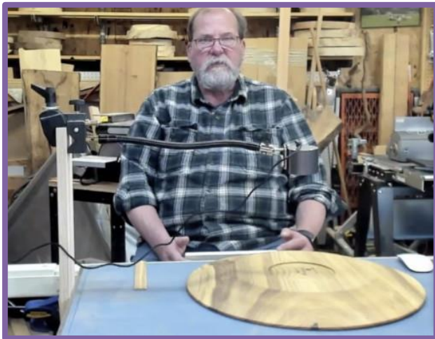
Dick also has a Laserpecker, but he has added a flexible gooseneck holder for the engraver
