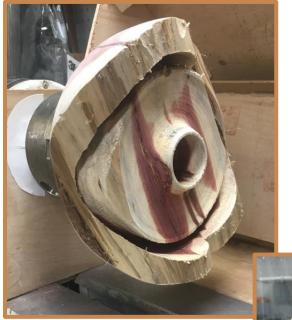
Red cedar NE bowl. I think we all do these a little differently. I like to use the parting tool to define the wall thickness all the way down to the low-side wall. Then I define the depth and eliminate the center with a Forstner bit.
