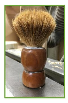
We need to get rid of sawdust/sanding dust all the time. Many of us do not have an air compressor system; using cans of compressed air is too expensive and not really very convenient. I've found the very best brush for cleaning my turnings is a shaving brush, fine bristles, easy to pick up, easy to keep within close reach.
