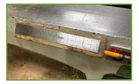
I got this tip several years ago and use it multiple times for every turning. The pencil is ALWAYS right at hand and a ruler that does not have to be picked up and held works so well for so many things. This is a triangular piece of scrap wood attached to the lathe with silicone glue/adhesive caulk.
