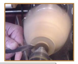
Before reversing the bowl cut a tenon for mounting in the chuck
