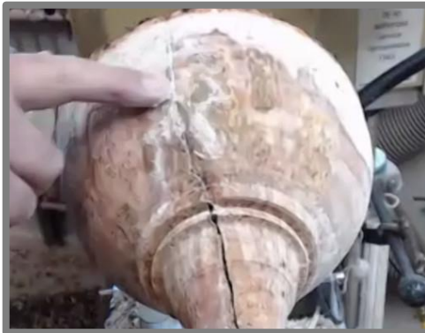
Adding sawdust to glue in crack
