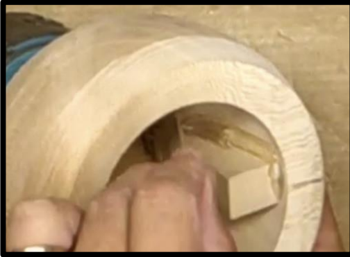
Dowel blocks held in place with hot glue
