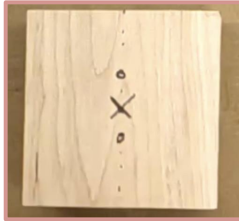
Holes for positioning dowels marked in what will be the center of the bowl
