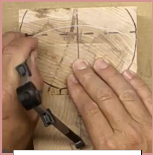
Compass centered on extension marks radius
