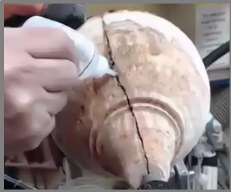
Applying medium CA glue to repair a crack in the bottom
