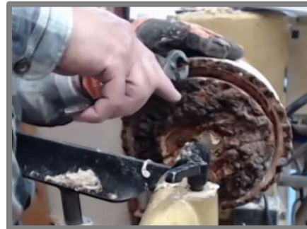
Clipping bark so it doesn't tear in turning
