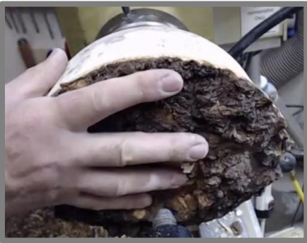
Bottom of bowl is finished; mount in chuck
