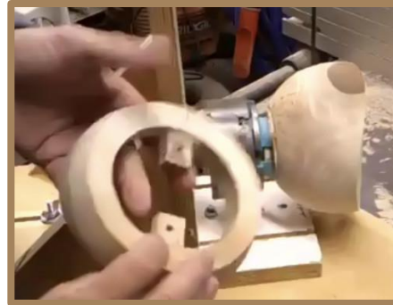
Top removed – note dowel blocks
