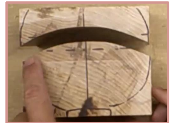
Aligning dowels planned so they will go through the top and into the lower portion of the block
