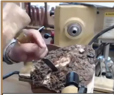
Clear bark so the wood can be mounted using the drive center
