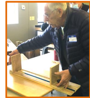
Dan Ernst-jigs for bandsawing big pieces and logs
