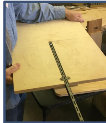
Glenn Anderson-jigs for handling large pieces for cutting
