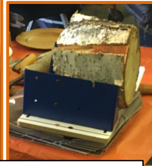
Dan's jig for safely x-cutting a log
