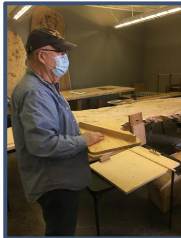
Glenn Anderson-jigs for handling large pieces for cutting
