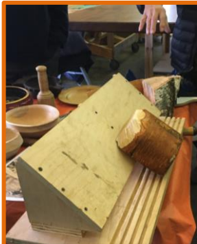
Dan Larson shows a jig for angling edges of logs before turning a bowl. Also, material from North House Folk School
