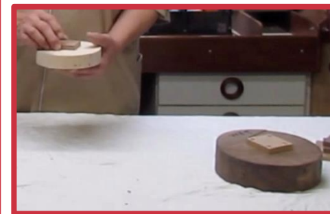
Jim screws the square on wet wood and glues it on kiln-dried wood
