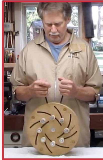
A Longworth chuck - homemade
