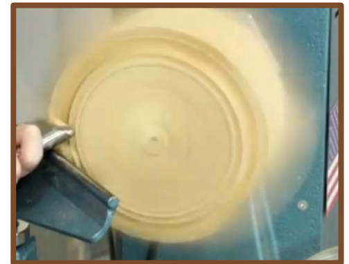
Beginning to turn the tenon and base
