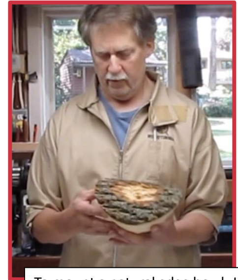
To mount a natural edge bowl, Jim clears away enough bark to get to solid wood and uses a 2-prong drive
