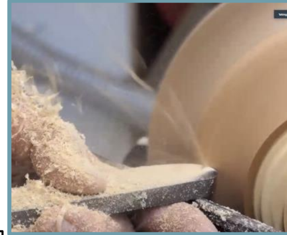
Scraper in action getting FINE chips
