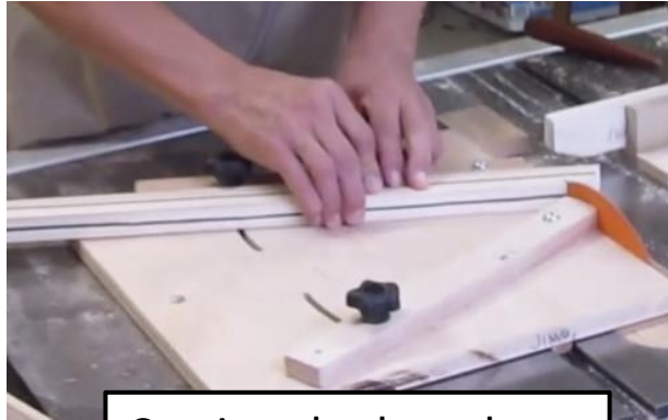
Cutting the length at the exact angle
