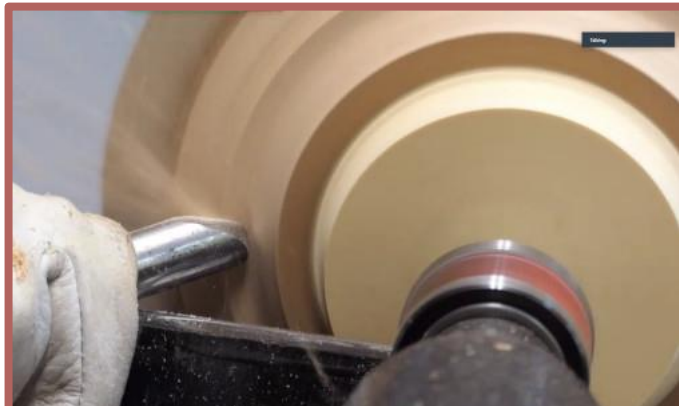
Glue block supported with tailstock as bottom of bowl and rim are turned
