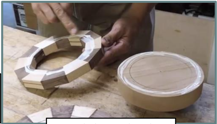
Spread glue on bowl blank and segment ring
