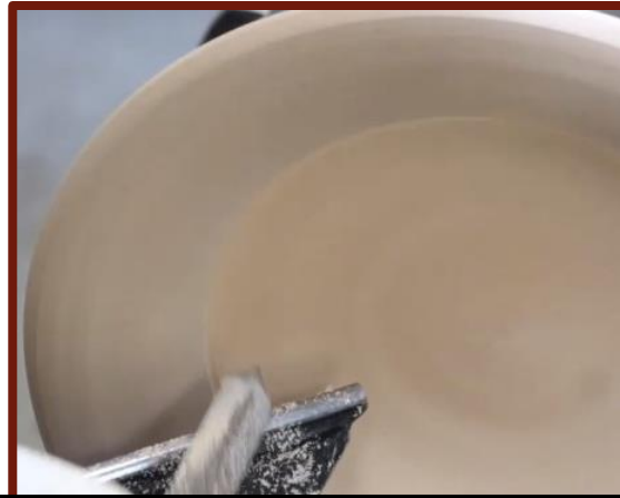
Corner of bedan tool demarcating rim from bowl; if there is later movement, this will disguise it
