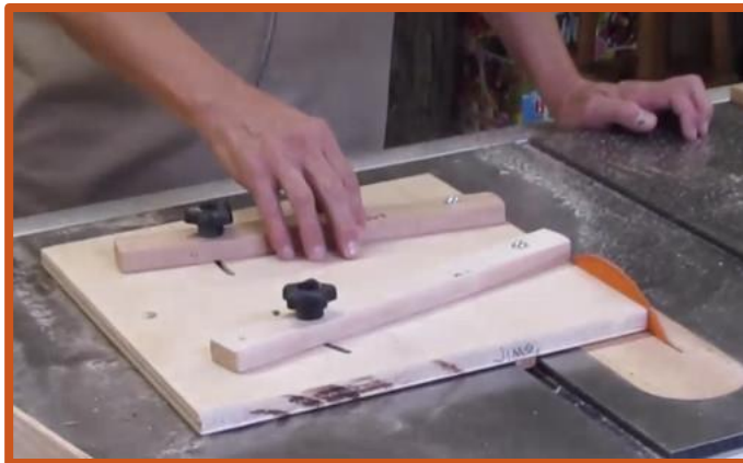
The 1 st cut will trim the edge of the sled
