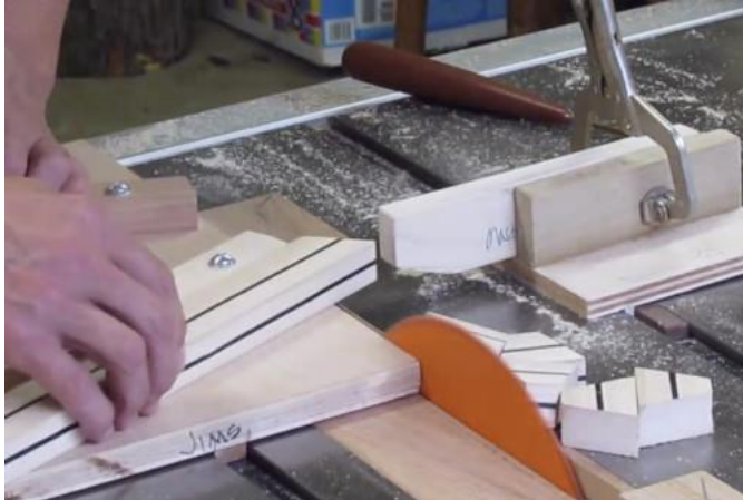
Segments being cut
