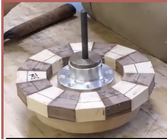
Attaching faceplate. Make sure screws are not too long for the bowl.
