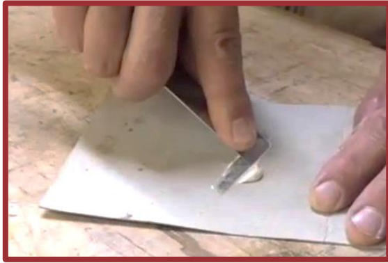
Final step in sharpening is using compound on cardboard
