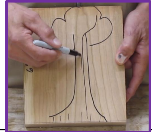
Jim draws a tree on the grain of a board to emphasize turning tactics depending on grain direction
