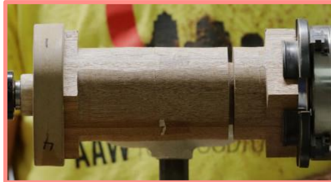
First cuts setting depth at critical points
