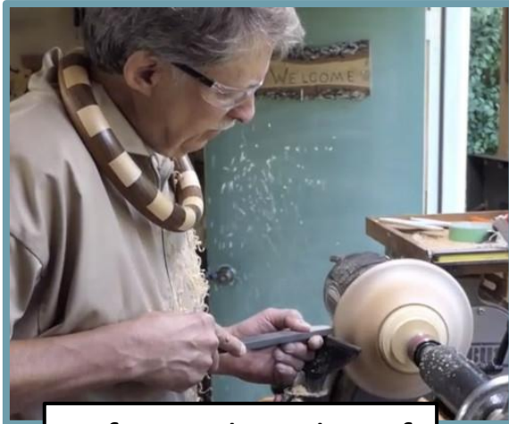
Refining the edge of rim with a scraper
