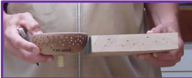
End grain is like straws going in one direction through the wood
