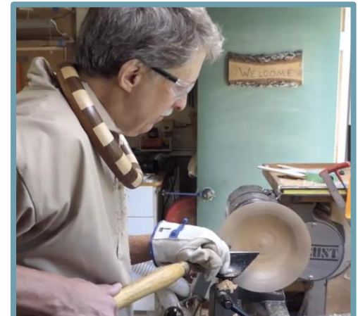
Finishing inside of bowl; tool against his body
