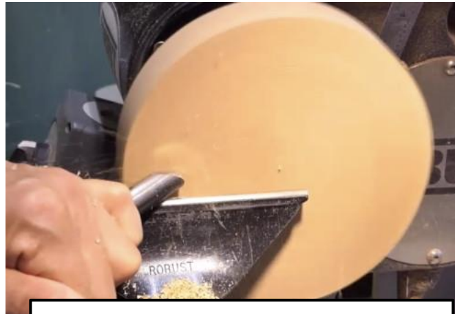
Pull cut, handle angled down, to true the face of the bowl blank
