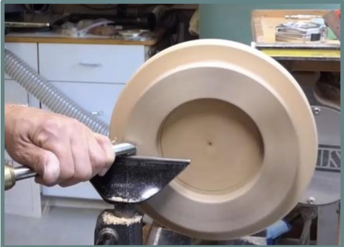
True the ring with LIGHT cuts
