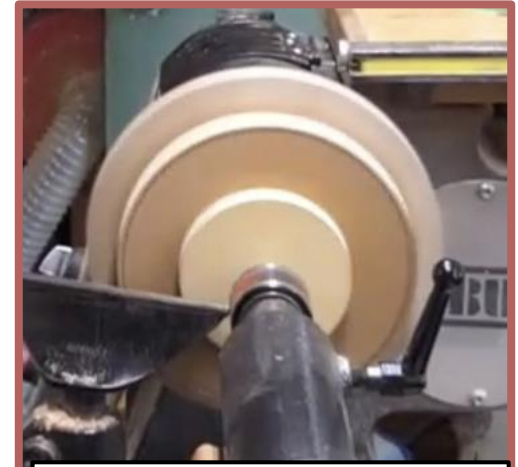
Glue block attached to bottom of the bowl
