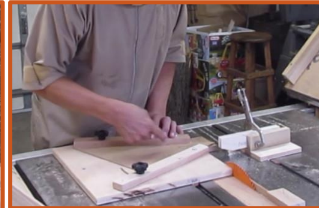
Adjustable stop is wedged very tightly into place
