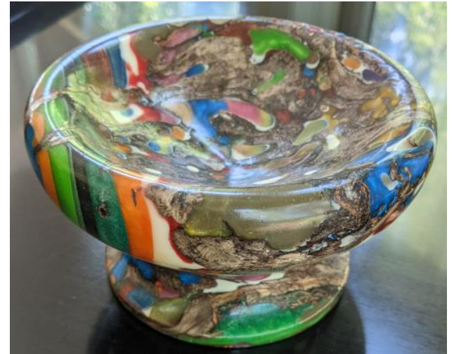
Honeycombed wood stabilized with different colored resins one at a time. Wood weighed 4 oz; finished piece weighs 4.7 lb.
