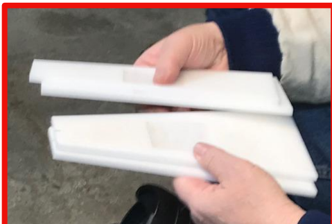
Wedge templates help align the guide arms on the Wedgie Sled
