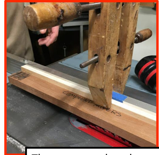
The compound angle template runs against this fence
